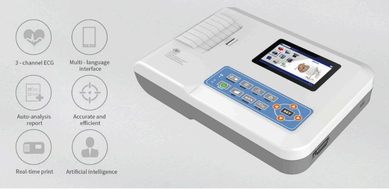
ECG300G is an Electrocardiograph which can collect 12-lead ECG signal simultaneously and print waveform by thermal printing system. It features in, recording and displaying ECG waveform in AUTO/Manual mode, measuring and diagnosing ECG waveform parameters automatically, prompting for "Lead off" and "Lack of paper", multi-language interface, AC/DC, optional rhythm lead that convenient to observe abnormal heart rhythm, case database management, etc.
